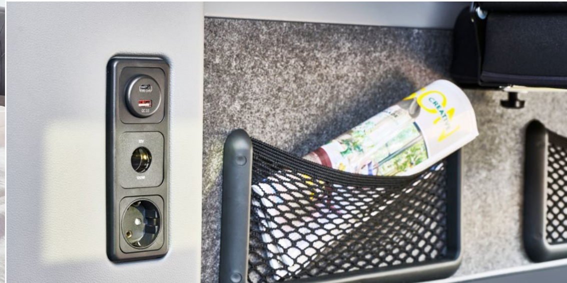
230V external socket, USB sockets also in the pop-up roof
